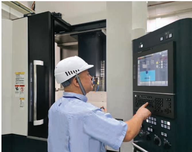
Easy operation with precise hand-eye coordination, aided by the 180° swing-type operation panel.
