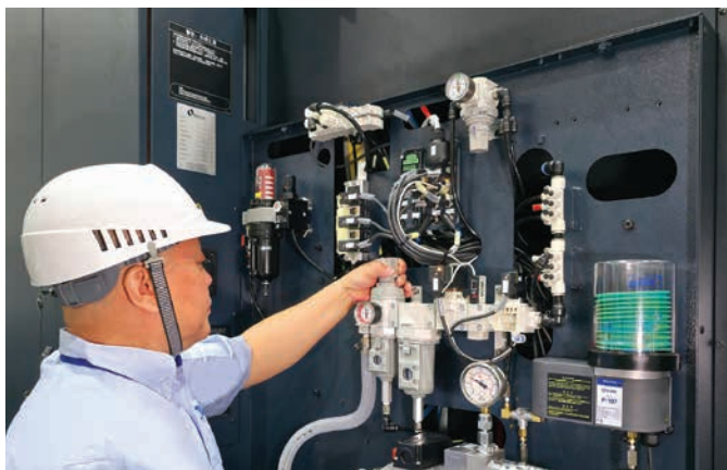
A centralised maintenance panel groups pneumatic, hydraulic and lubrication points for quick and efficient servicing.
