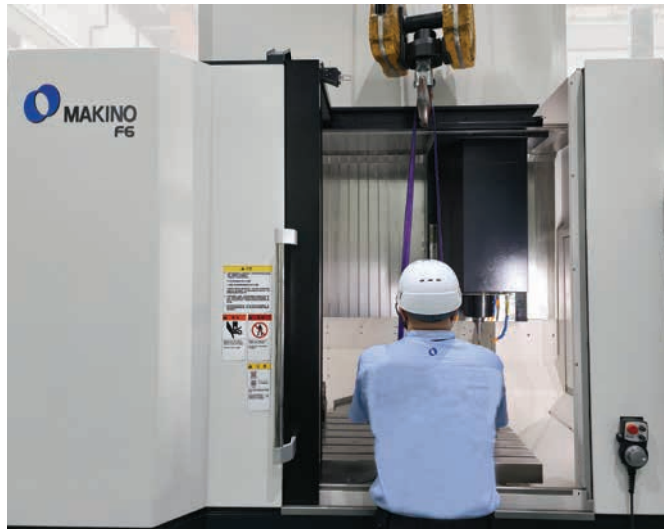
The machine ceiling opens to allow easy handling of large, heavy workpieces and fixtures using an overhead crane.
