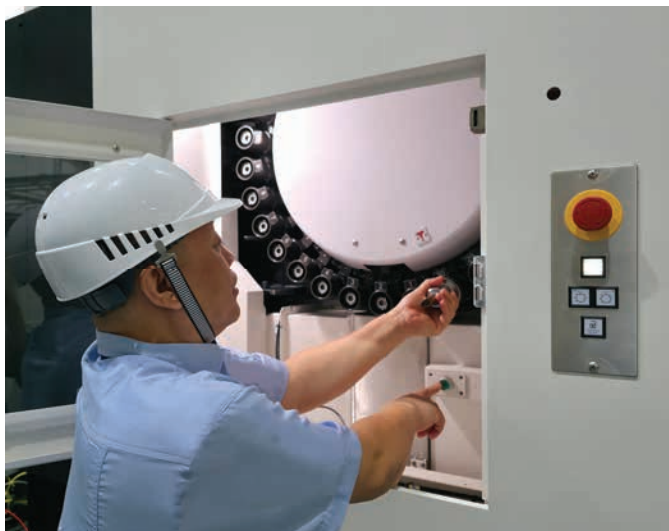
Convenient ATC magazine access for tool loading/unloading, supported by an unclamp/clamp push button.
