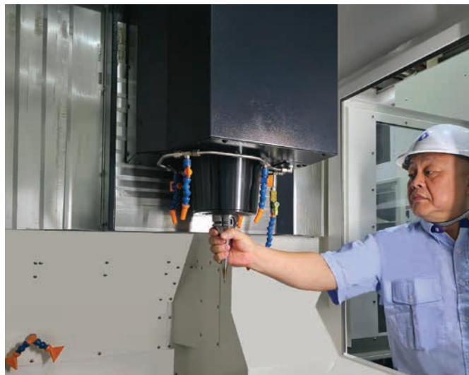
Side door access enables easy spindle approach for tool changes.
